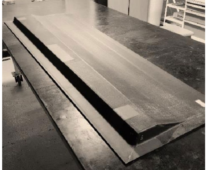
Aramid Honeycomb & Carbon Fiber Spoiler
