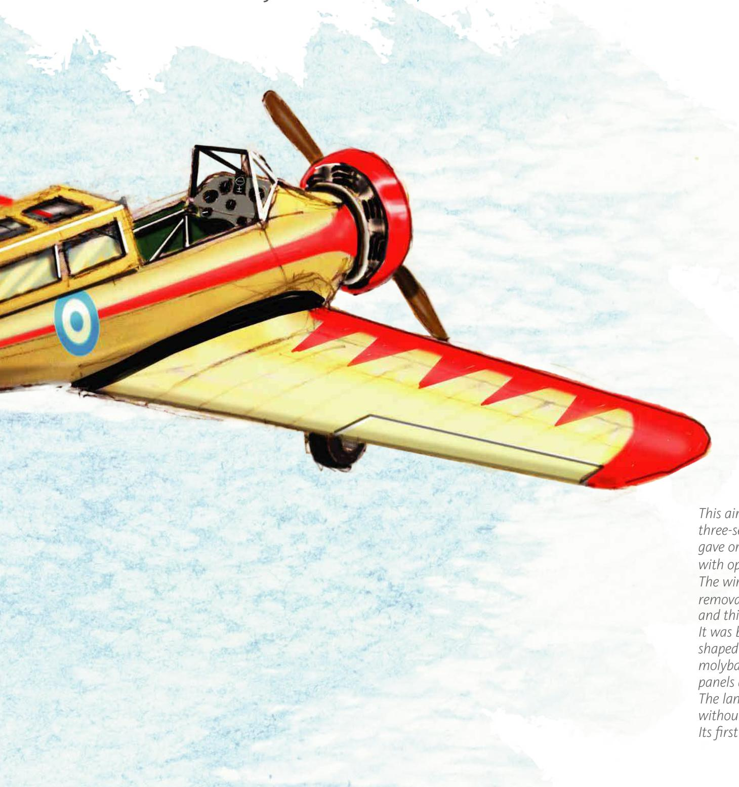
This aircraft was a low wing cantilever monoplane, three-seater aircraft with closed cockpit, which in later gave origin to a single-seater and a two-seater aircraft with open cockpit.
