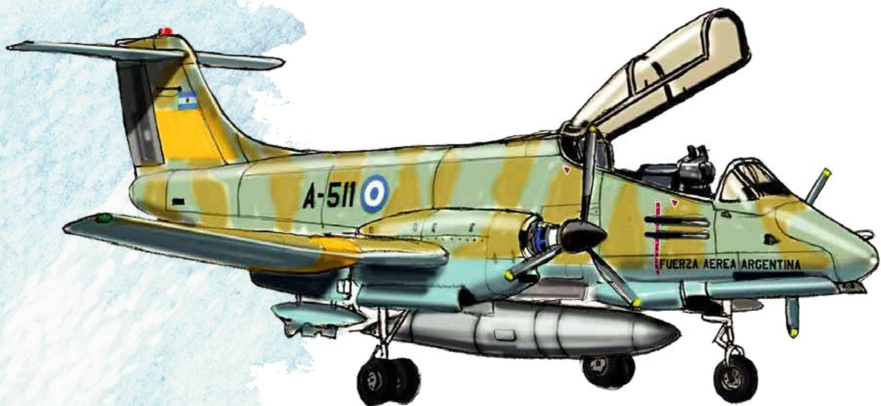
A metallic cantilever low wing twin engine aircraft specially designed for COIN and attack missions. During Malvinas War it proved to be an effective "helicopter hunter". Its first flight took place on August 16, 1969 powered by two turboprop 904 hp thrust TPE Garret engines. Later on, serial aircraft were equipped with Turbomeca Aztec XVI-G. Initially, it was designed as a twin seater but after Malvinas war a one-seater version was developed,
